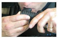
Release the pressure on the dump button before removing your mouth from the mouth piece.
