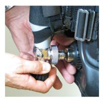
2. Remove the rescue air inflation cylinder by unzipping it from the BC.
