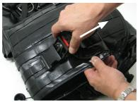
2 Load the weight pockets with an appropriate amount of weight and close the velcro flap on the pocket.
