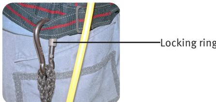
3. Check that the air supply hose is pressurised. Connect the quick coupling on the P+ regulator to the breathing apparatus. For versions with Interspiro quick connection, lock it with the locking ring.
